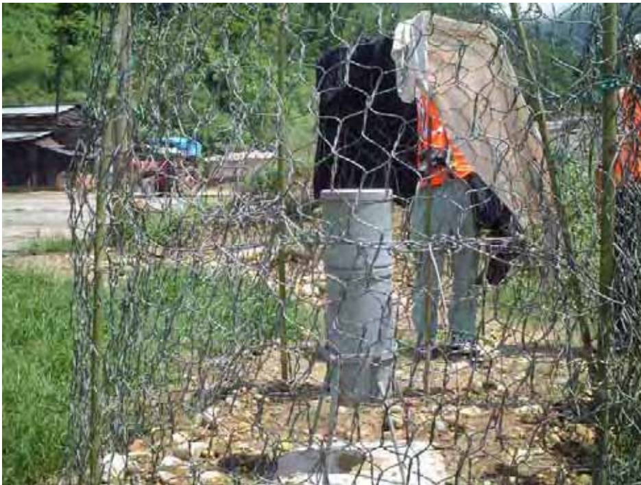
Figure 2.3.6 Rain gauge station at Kahare Kohola
