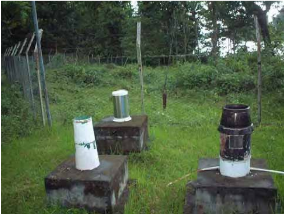
Figure 2.3.5 Rain gauges at Devigaht Station
