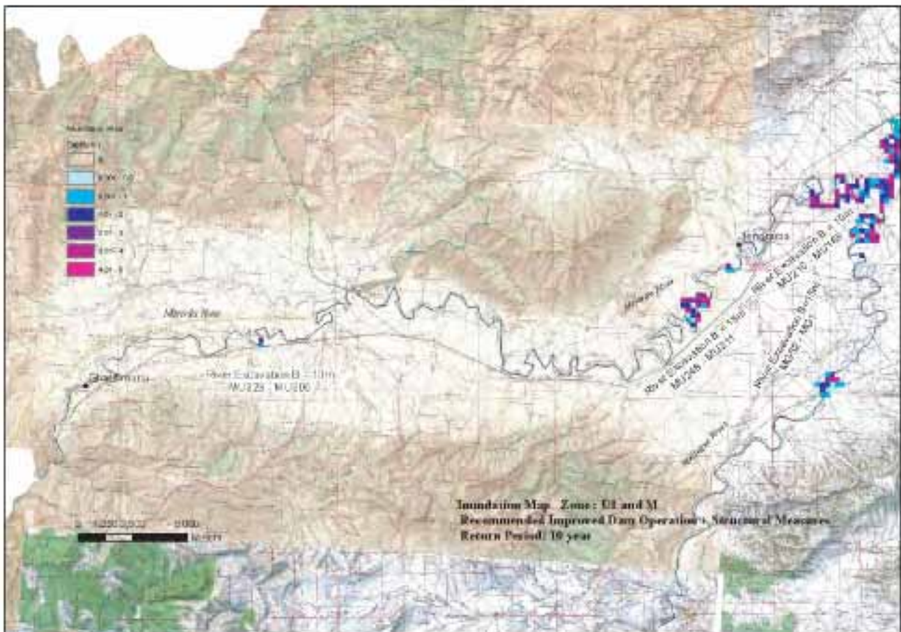
Inundation Simulation Result Recommended Dam Operation 2030 + River Improvement: Zone U1 (1/2)
