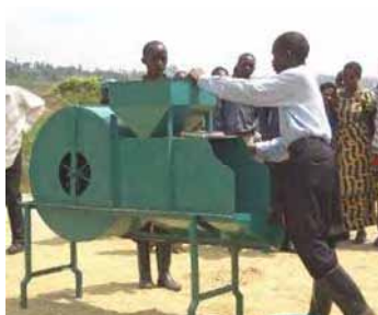
The agronomists demonstrated how to operate winnowing machine on the newly constructed drying yard
