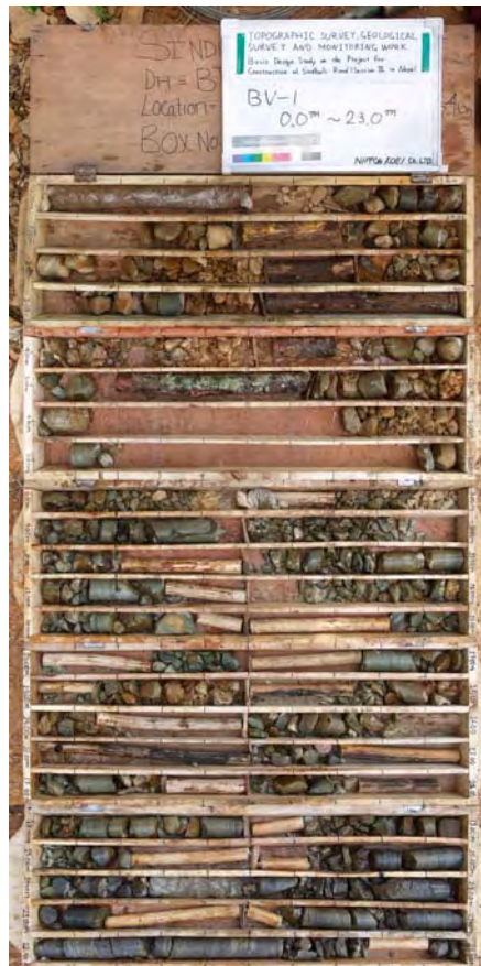
Photo 6-6-1 BV-1 bore core photograph
