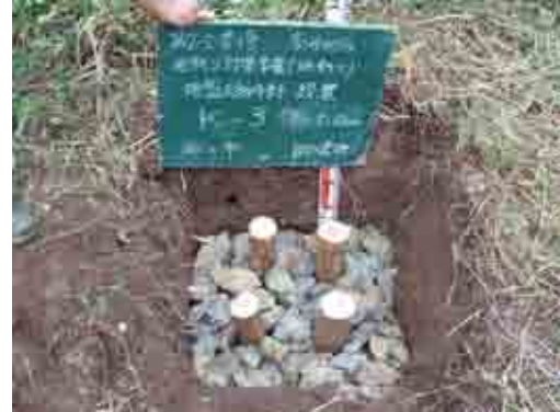
Picture: Process of setting a tilt-meter
