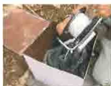
STEP5: Drop the sensor. When the sensor touches with Groundwater, extend a buzzer.
