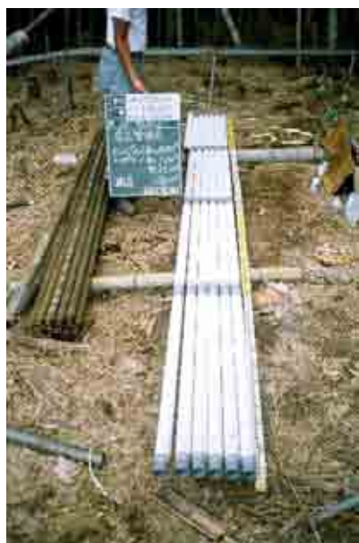
Picture3.1 Process of setting the pipe strain gauge
