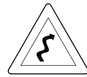
WINDING ROAD W 1-5
