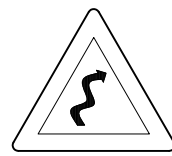
WINDING ROAD W 1-5
