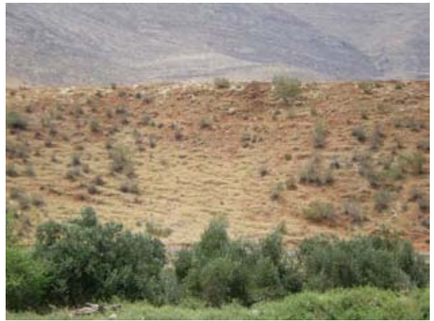
Ph-F18, F19 Reddish top soil around here deems to be suitable as an impervious core.
