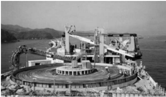
Length and weight of cable coiled around turntable: 50km, 5,000t
