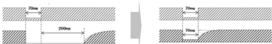
(a) Control Method of Conventional DC system In case of AC voltage drop, DC system needs to stop and restart and it takes over 200ms until restore power. (b) Control Method of Latest DC system In case of AC voltage drop, Dc system enables to be operated continuously. So, reliability is the same as AC system
