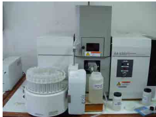
Photo 6.2.4 AAS-Shimadzu6300 (flame type)
