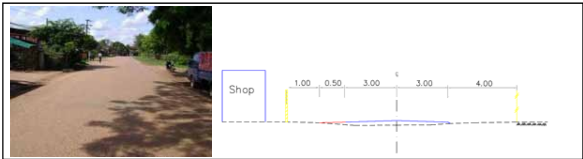
Figure 25.4-6 (2) Present University Road Condition: (KM 0+450) RW=9~12m
