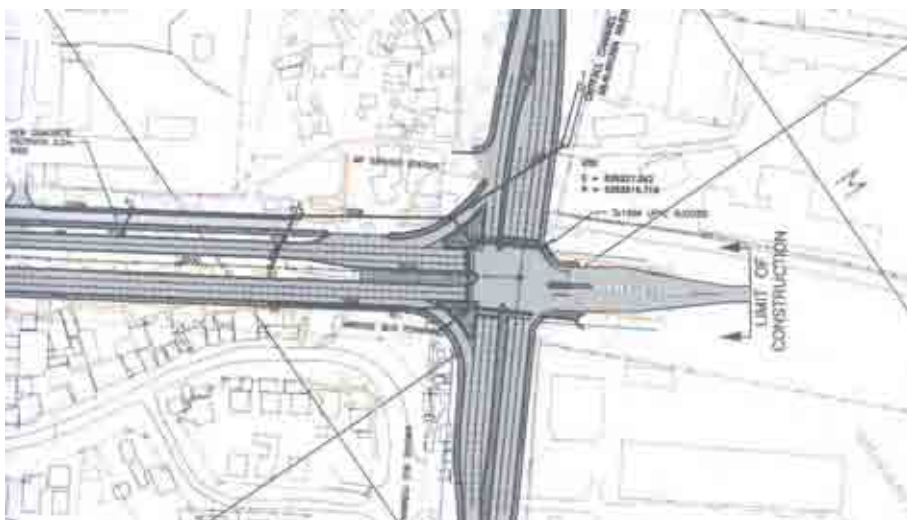
Figure 5.3.3 Improvement of Mwenge Intersection in Sam Nujoma Road Widening Project
