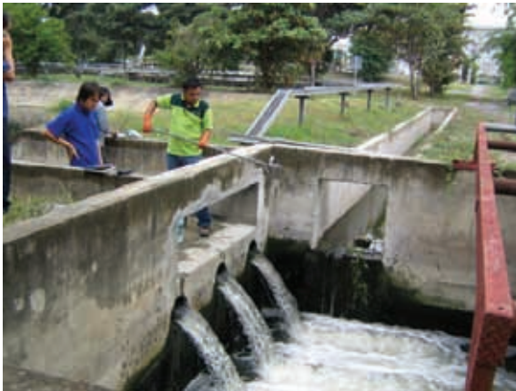
Sampling at the wastewater treatment center outlet of Suan Autasahakham Rojana Industrial Zone, AYP.
