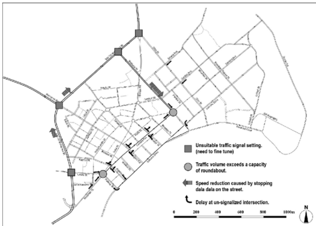
Figure 2.3.23 Problems of Existing Traffic Flow in 7:00 – 8:00
