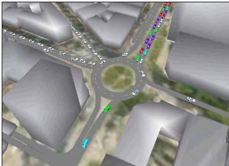
Figure 7.2.2 Simulated queue build-up at Askari Monument Roundabout indicating over-capacity conditions
