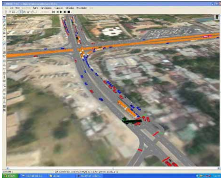
Figure 5.2.11 Queue Build-up along Sam Nujoma U-turn Facility Simulation of BRT Phase I Base Case
