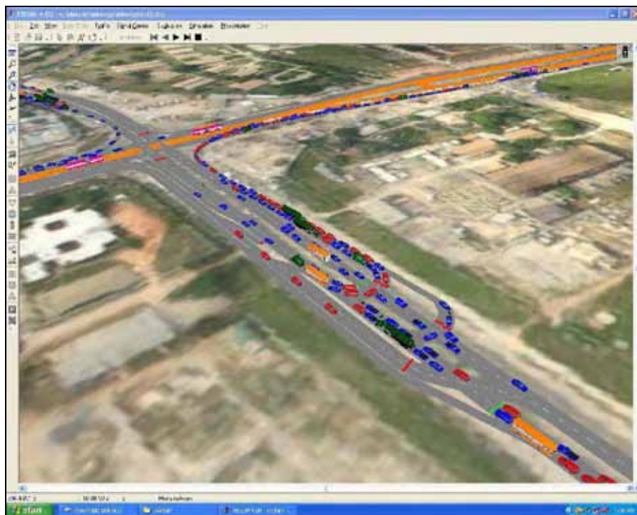
Figure 5.2.12 Queue Build-up along the Nelson Mandela U-turn Facility Simulation of BRT Phase I Base Case
