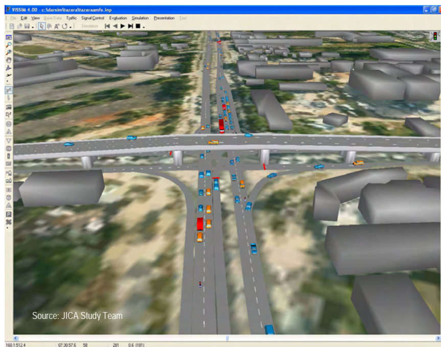
Figure 2.1.2 Flyover Provided for Nelson Mandela Road Simulation of Existing Peak Period Condition
