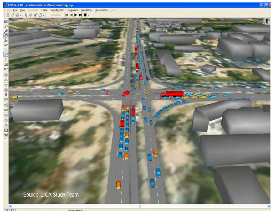
Figure 2.1.1 Queue Build-up along Nyerere Road Approaches Simulation of Existing Peak Period Condition
