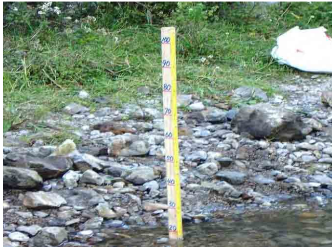
Photo III-3.5.1-9 after Installation of Staff Gauge (ST.1)
