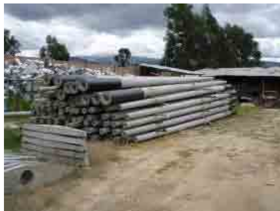
<Pole (High Voltage)>
