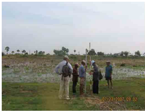
JICA study team trained simple survey for reservoir to prepare H-V curve
