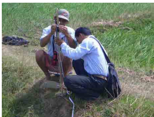
PDOWRAM counterparts set a current meter for canal discharge measurement.
