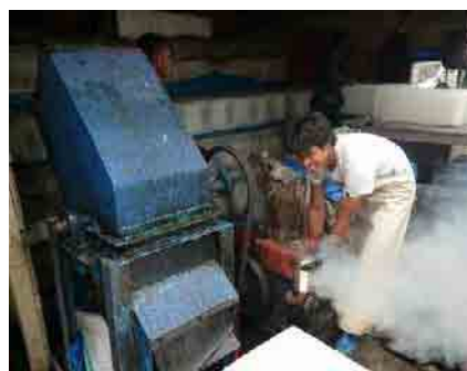
Block Ice (L) and Diesel Engine Driven Ice Crushing Machine (R)
