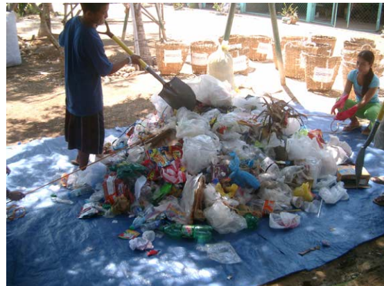
Mixing in the Process of Quartering Method of Solid Waste (March, 2007)
