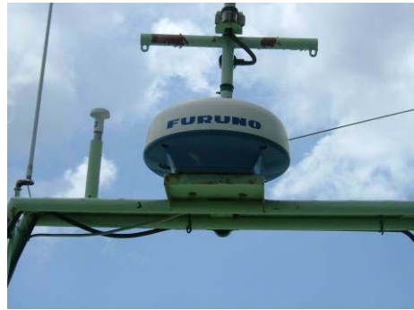
Photo 5-8: Radar Scanner installed on the Wooden Boat
