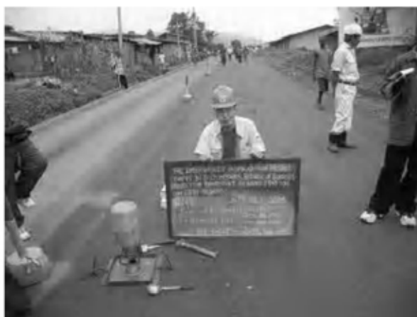
Date : 26 , 29 , 31/1/2008 Activity : RN7 Base Course Quality Control Field Density Test Sta.-0+025 ~ 1+060 Right Side
