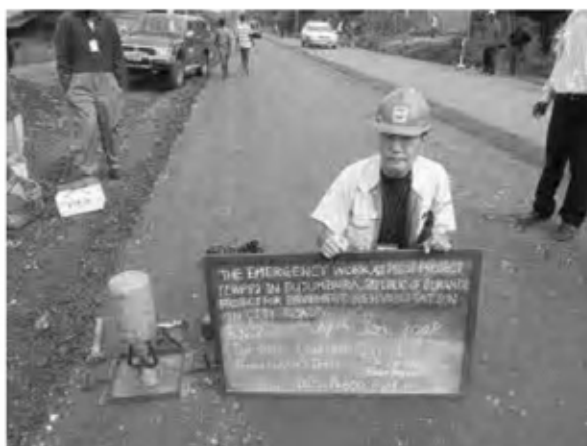
Date : 18, 19, 24, 25/1/2008 Activity : RN7 Sub-base Quality Control Field Density Test Sta.-0+025 ~ 1+500 Right Side
