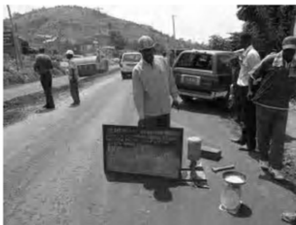
Date : 9/1/2008 Activity : RN7 Sub-base Quality Control Field Density Test Sta.1+500 ~ 1+660(EP) Right Side
