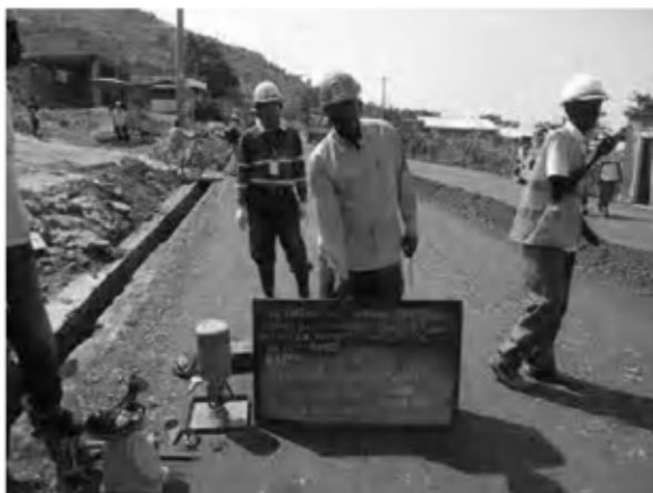
Date : 9/1/2008 Activity : RN7 Base Course Quality Control Field Density Test Sta.1+500~1+660(EP) Left Side
