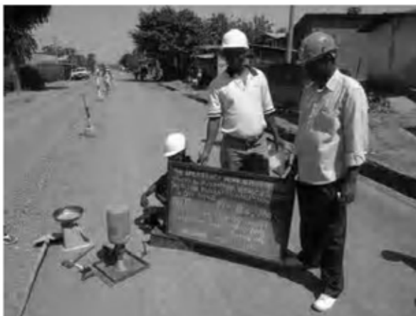
Date : 11 , 14 , 17 , 20/12/2007 Activity : RN7 Base Course Quality Control Field Density Test Sta. -0+025 ~ 0+240 Left Side Sta. 0+280 ~ 1+500 Left Side
