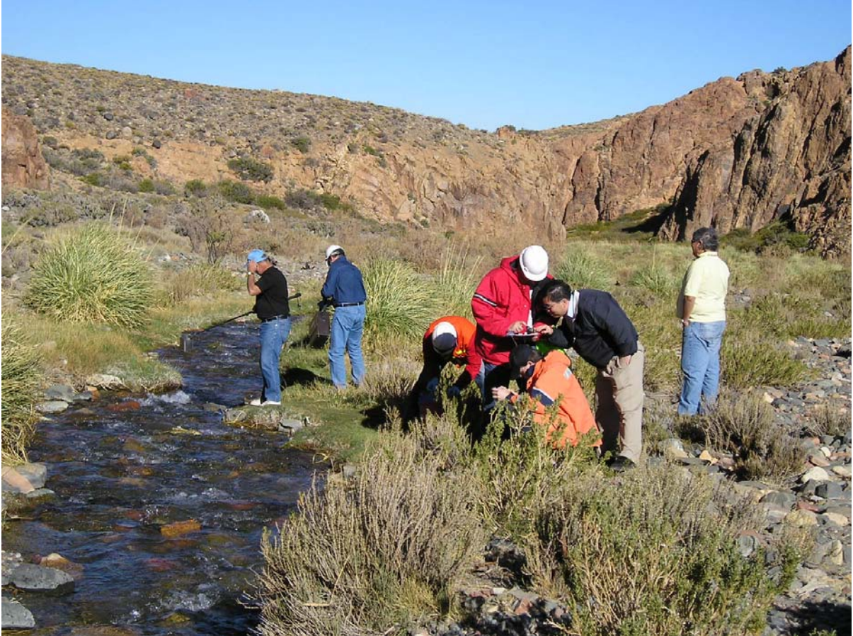
Taking a sample of mine waste downstream water in Arroyo Conconta
