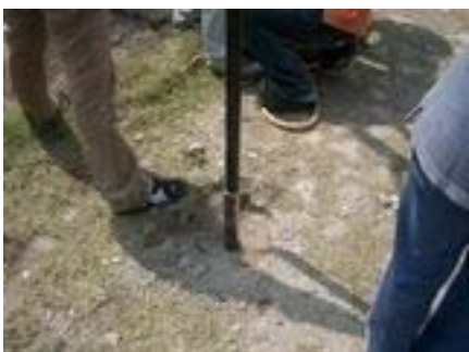
Standard Penetration Test (Collecting Sampler)
