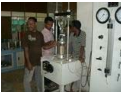
Tri-axial Compression Test (Shearing of Specimen)
