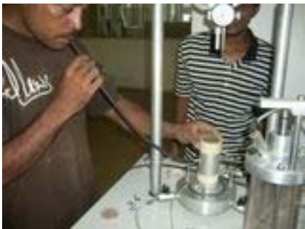
Tri-axial Compression Test (Setting up Specimen)
