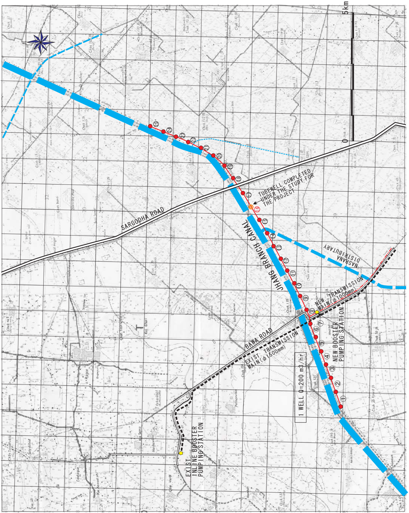
FIG. 2-10 LAYOUT OF TUBEWELLS ALONG JHANG BRANCH CANAL
