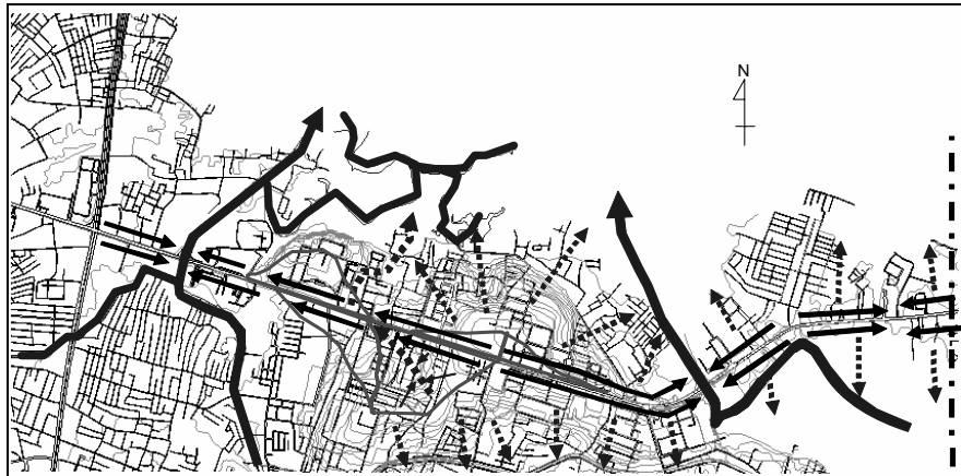
Figure 7.10.19 Existing Drainage Network of Section A (1/4)
