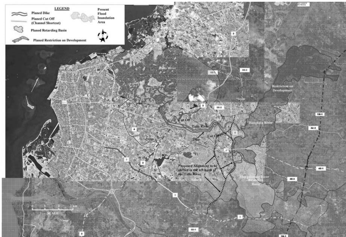
Figure 6.1.4 Flood Inundation Area, Flood Control Plan and Proposed Road Alignments in the Tallo River Basin
