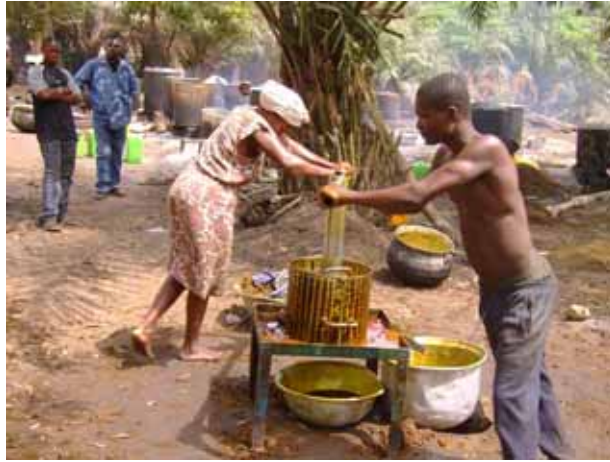
Figure 2.2-6 Manual Screw Press with Short Effort Arm
