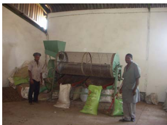
Grading machine for cashew nuts
