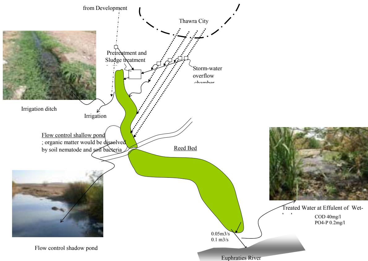
Figure A9.3.6 Schematic Plan of Wet Land in Thawara
