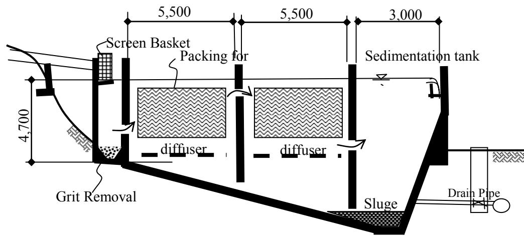
**Figure A9.3.1 Schematic Section of Slunfeh STP**
