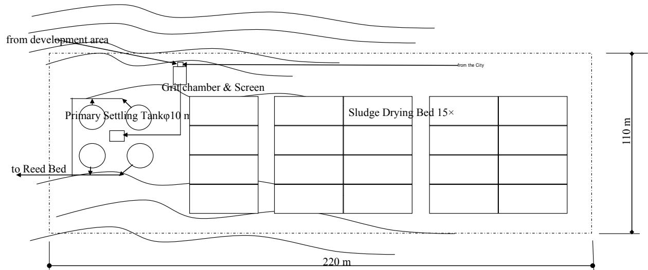
Figure A9.3.7 Layout Plan of Pretreatment and Sludge Treatment Facilities in Thawra STP
