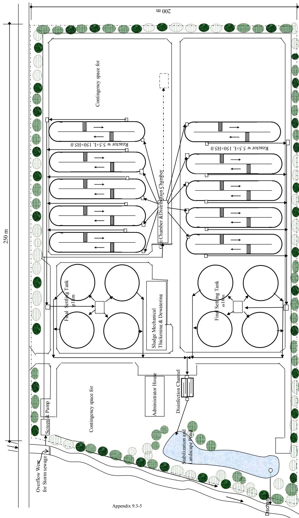
Figure A9.3.9 Layout Plan of Zabadani STP
