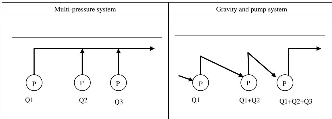
**Figure A9.5.1 Pattern Diagrams of Two System**
