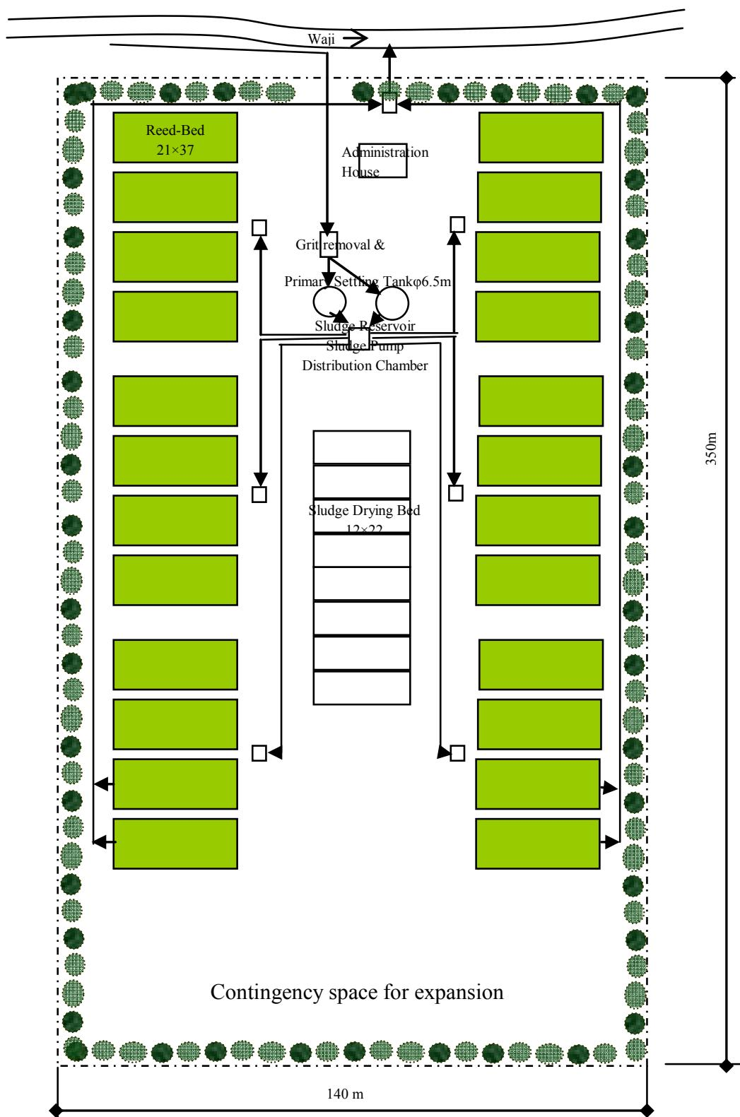
Figure A9.3.8 Layout Plan of Muzerib STP
