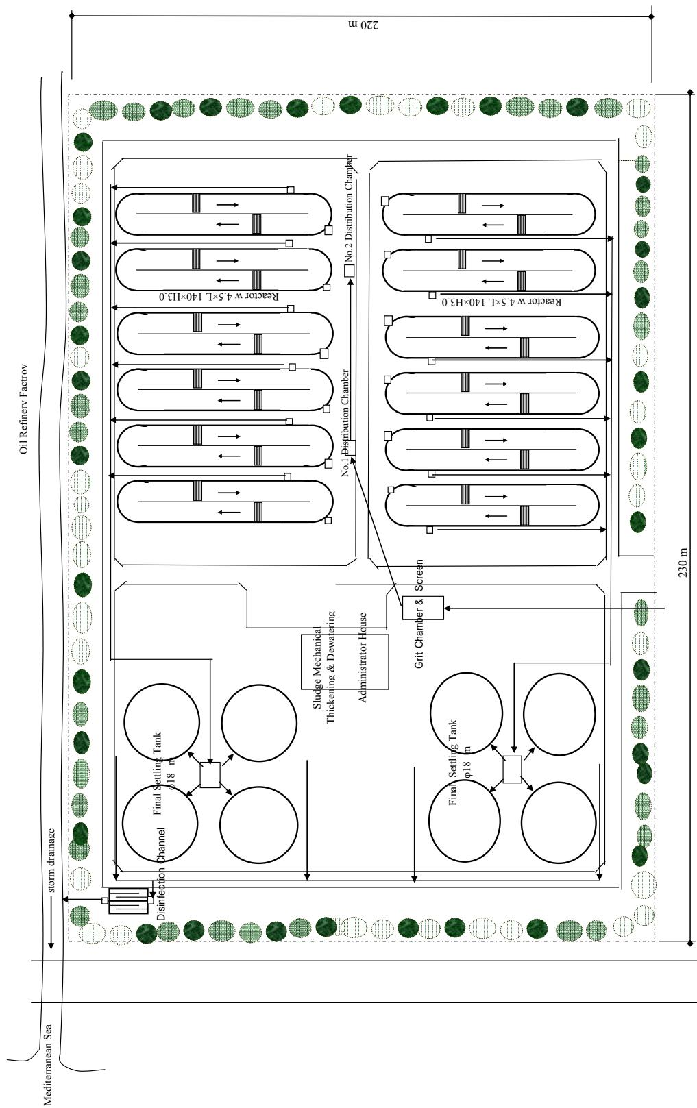
Figure A 9.3.3 Layout Plan of Banias STP
