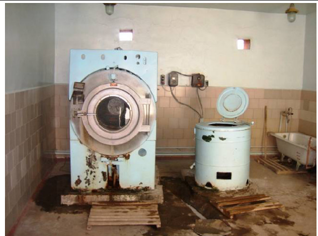
Washing machine and extractor
