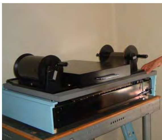
Figure 3.2.4 Scanning of a roll film by Ultrascan 5000
