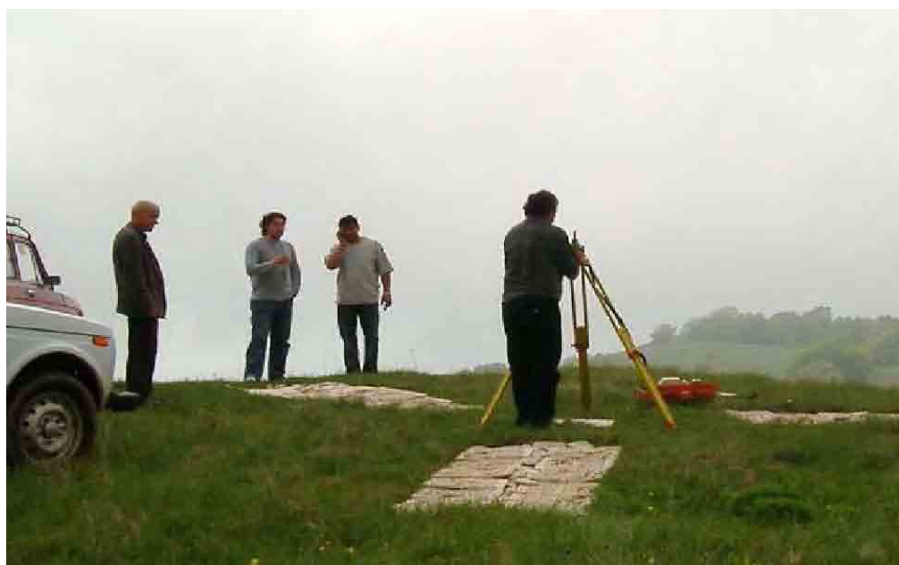
Figure 3.3.2 Observation of GCP in the field
