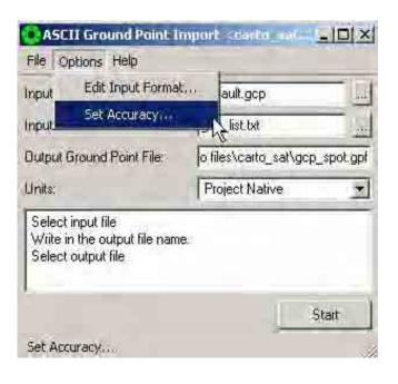
10. A "Set Accuracy" dialog box will appear. Type "7" in "X Accuracy" box, type "7" in "Y" Accuracy" box, and type "10" in "Z Accuracy" box. The values are the handheld GPS accuracy level in XYZ. Then click "OK".
