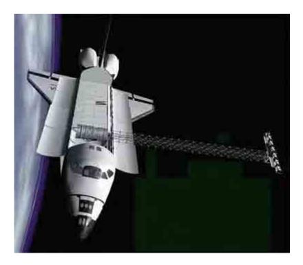
Artist representation of SRTM in space. Main antenna is located in the payload bay, the mast is deployed to 60 meters (200 feet), and the outboard antenna is attached to the end of the mast. (Courtesy of the German Aerospace Center)
