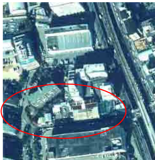
Local distortion of a road (example of an aerial photograph)
