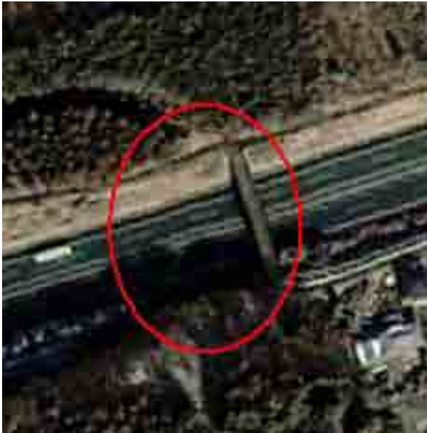
Local distortion of a section of a road (IKONOS Satellite Image)
