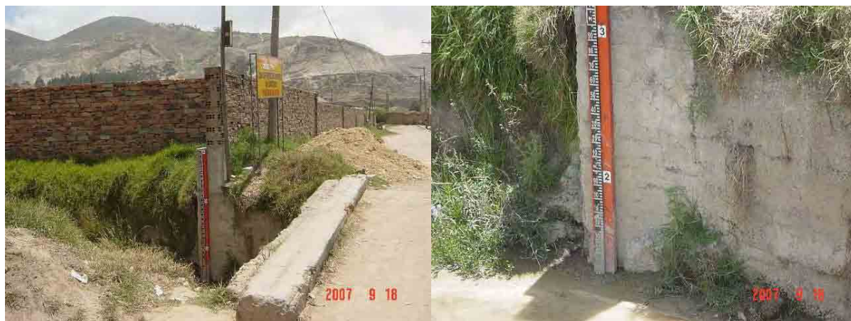
Photo S8-2-19 Water level gauge at Llano Grande
