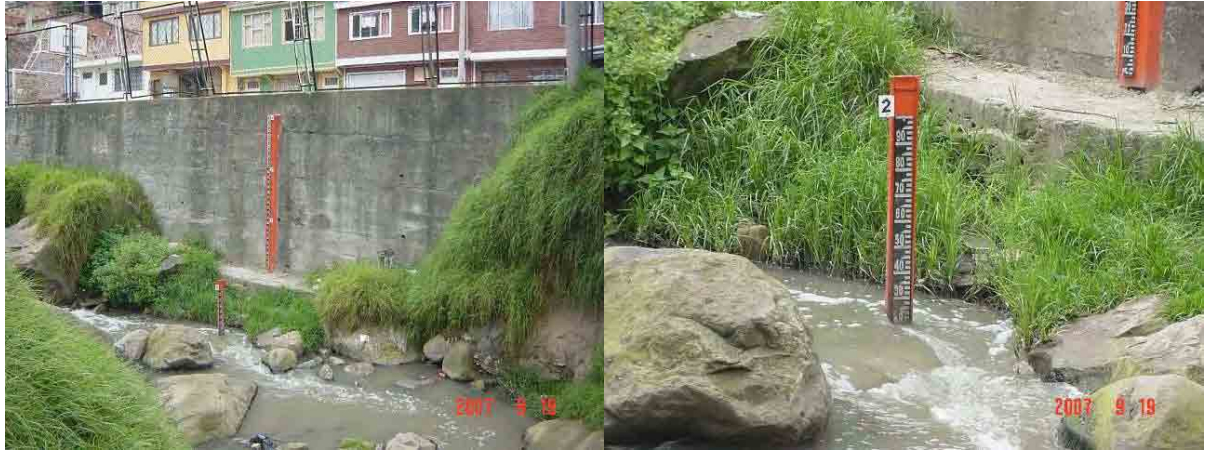
Photo S8-2-4 Water level gauge at La Gloria
