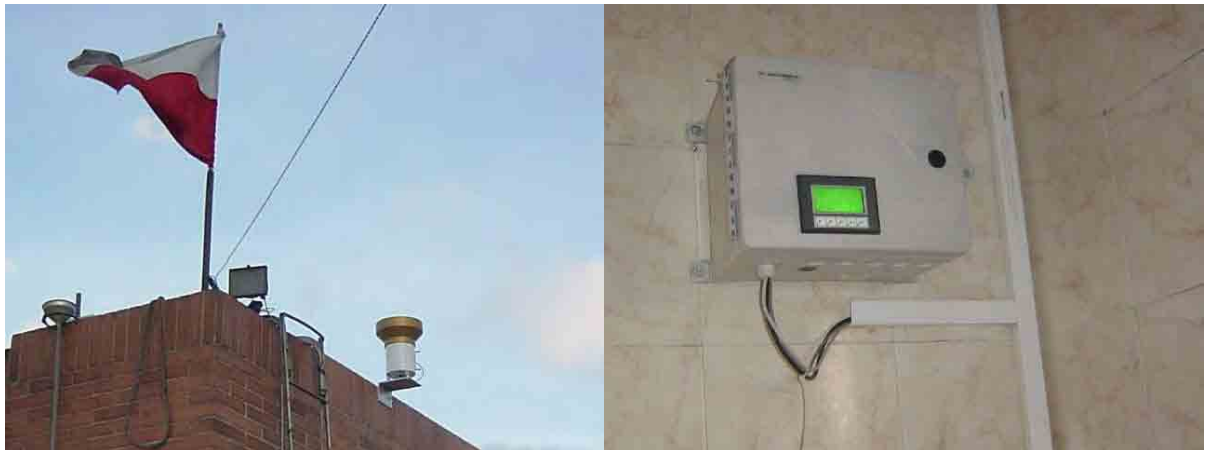
Photo S8-2-12 Rainfall Gauge and Data logger
