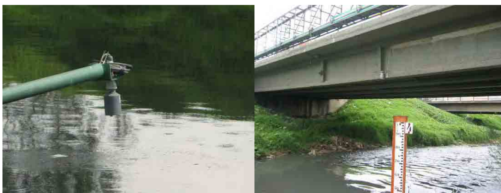
Photo S8-2-2 Non-contact stage measurement sensor (left: EAAB La Isla Station, Bogota River, right: DPAE San Benito Station, Tunjuelo River)
