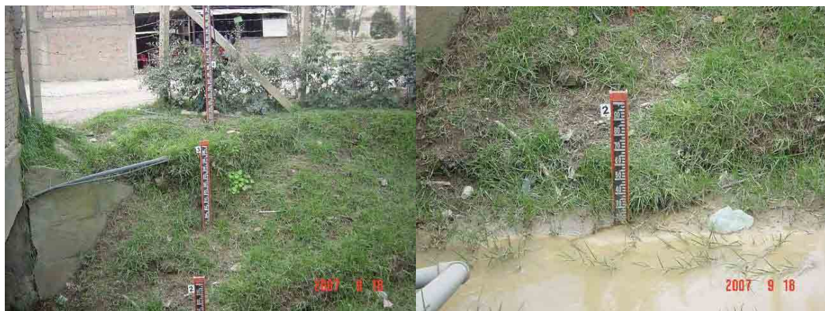
Photo S8-2-17 Water level gauge at Ladrillera Santa Fe
