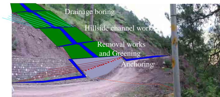
Figure 4.1.8 Typical counter measures against landslides in order to secure the definite stability
