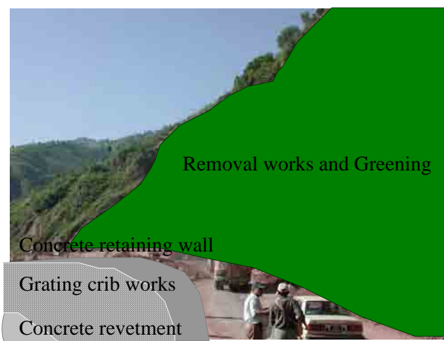
Figure 4.1.5 Recommendation of countermeasures against slope failures of toppled rock mass and overlying debris
