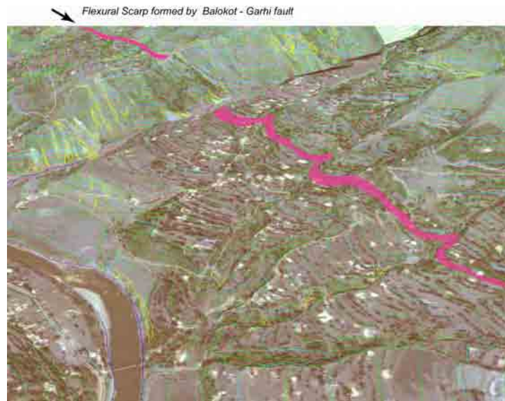
Figure 3.2.10 Flexural slope on the right bank of the Jhelum River around Totha downstream of Naushana
