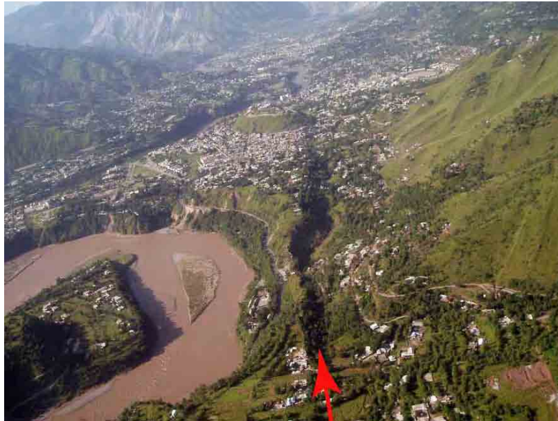
Photo 3.2.2 East facing active fault scarp of the Jhelum Fault south of Domei, Muzaffarabad
