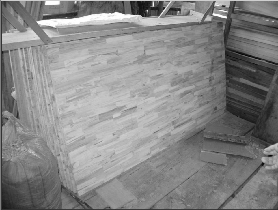
Photo No. 3.4 (Acacia) Laminated Finger Joint board (Lam Dong)
