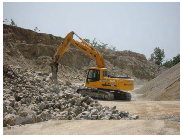
A large breaker made in Korea can move by itself to break large size limestones.
