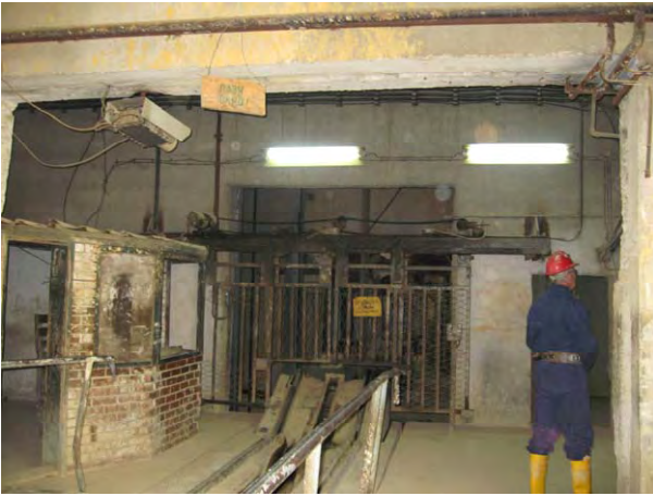
Cage to enter the underground. Its size is 4m × 4m with double-deck. The cage is linked with 500m deep from the surface.
