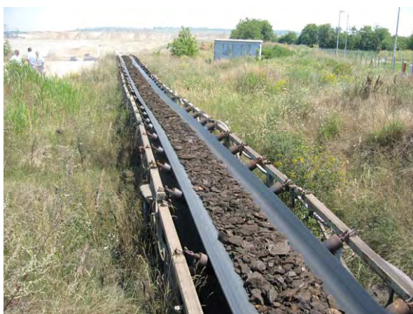
Mined coal is transported by belt conveyors to the generation plant.
