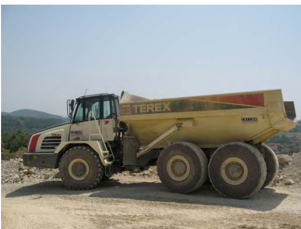
A dump truck transports blasted limestone to the the crushing plant.
