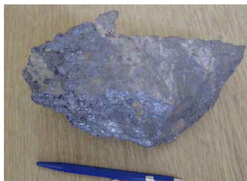
High-grade massive molybdenum ore in the Suva Ruda mine office. The area has high potential for mineral resources.
