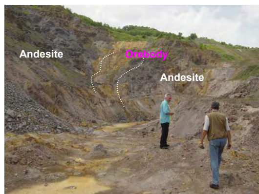
An open pit of the No.2 Ore Zone at the Kizevak deposit. Thickness of the orebody ranges from 7 to 10m.
