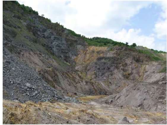
This orebody was mined without safety benches at the open pit. It seems over-mined
