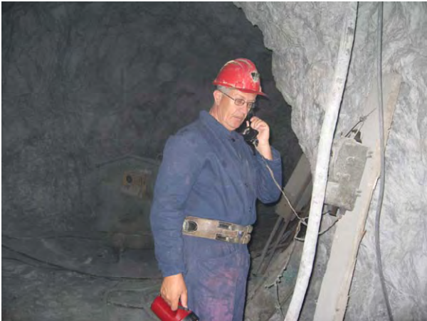
There a telephone nearby the working stope. Workers can communicate with the surface.
