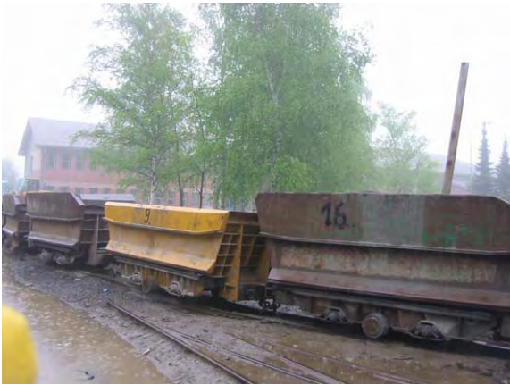
Mine cars transporting ore to the processing plant from underground at the 1,300m level
