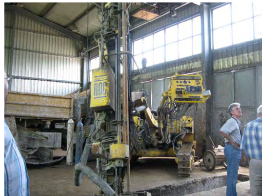
Several mining machines used in the pit. This photo shows a comparatively new drilling machine with a compressor.
