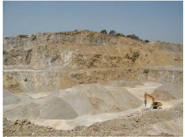
A pit bottom is used to store the products.
