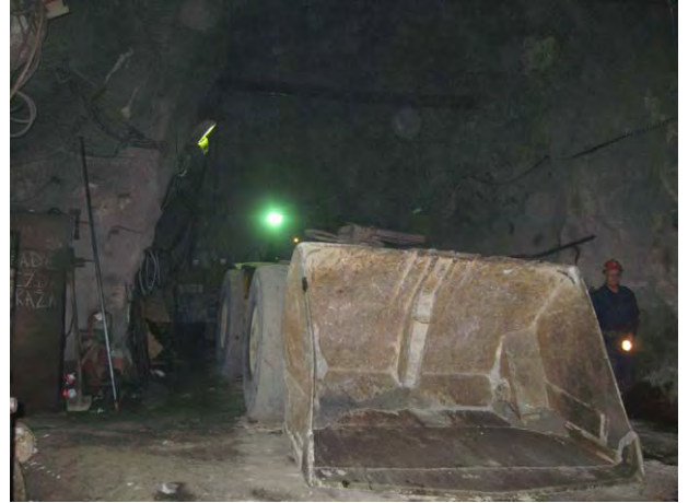
A transporting machine, LHD (ST-6) made in USA. This machine is parked in the underground pit.
