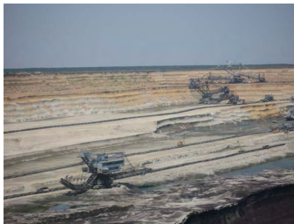
Continuous cutters are working to mine coal seams in the pit. Each cutter is connected with belt conveyors.
