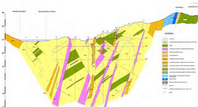
Fig.4.6 Geological Section of the Veliki Krivelj
