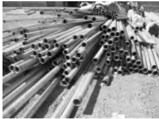
Galvanized Steel Pipe in Stock Yard
