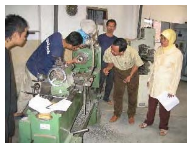
Measurement of a lathe’s precision on the shop floor
