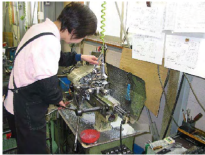
Drawings are posted in front of the operator so that she can check as necessary.
