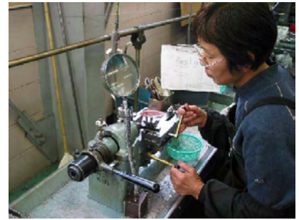
The magnifier is placed on the machinery so that the operator can check precision on sample basis. A calliper is also placed on the desk as shown in the middle photo.
