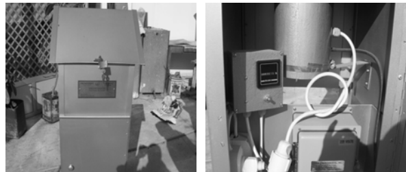
Hi-Volume Sampler to measure the (TSP)
