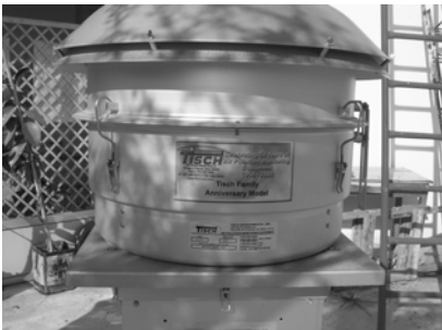
Hi-Volume Sampler to measure the (PM10)
